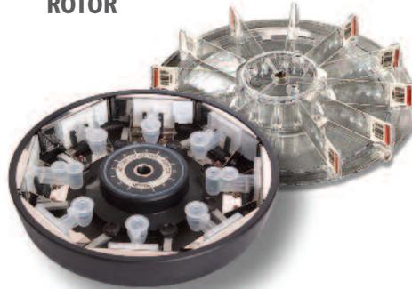
With the optional Cytopro® Rotor, the Aerospray Stainer becomes a superb cytocentrifuge with eight-slide capacity and programmability, at a fraction of the cost of purchasing a stand-alone cytocentrifuge.
